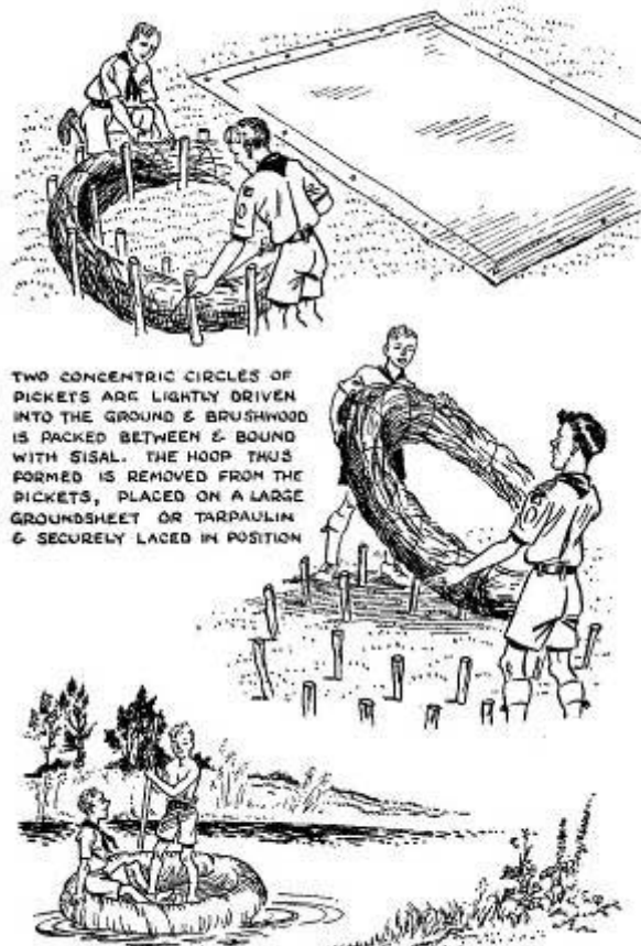
Coracle built from sticks and a groundsheet.
